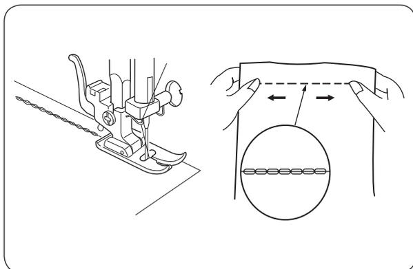
The stitch is sewn with two forward stitches and one reverse stitch, creating a seam that is difficult to tear.
