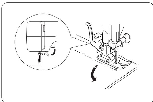
Stop the machine and turn the handwheel toward you to bring the needle down into the fabric.
