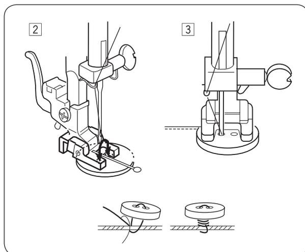
② Match the holes in the button with the horizontal slot on the presser foot.
